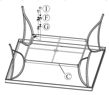
After making any necessary adjustments to the alignment of the table, use the hex bolt driver and hex wrench to tighten all bolts . **Note:** each bolt must be tightened a few revolutions at a time. In order to apply equal pressure to all bolt joints, we recommend working in a cross corner (X fashion). Repeat until all bolts are tight. **Do not over tighten.** Over tightening may strip bolts. Cover all bolts with covers.
